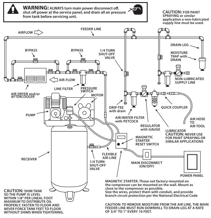
NOTE: RECOMMENDED PIPE AND FITTINGS: BLACK IRON PIPE no smaller than tank outlet size (NPT). For systems over 100 feet in length increase by one pipe size.
