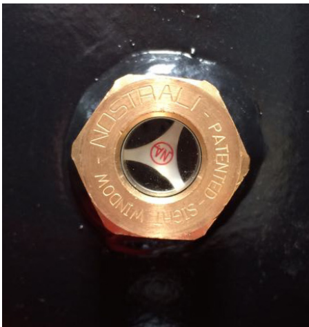
✗ Completely Empty Tank
