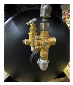
Pilot valves are factory pre-set for the optimum operating pressure. **DO NOT** adjust this valve. Adjusting this valve will void package warranty and can cause the premature failure of the compressor.
