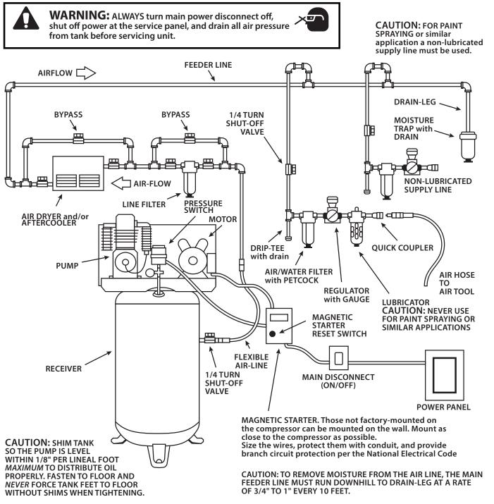
NOTE: RECOMMENDED PIPE AND FITTINGS: BLACK IRON PIPE no smaller than tank outlet size (NPT). For systems over 100 feet in length increase by one pipe size.
