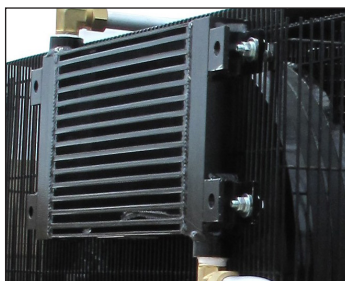
Air cooled after cooler Platinum unit
